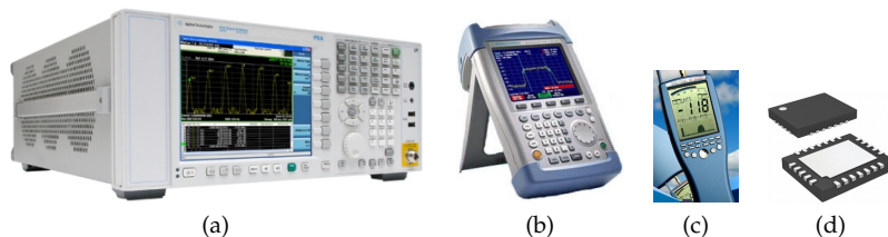
Figure 2.3: Examples of SAs (scale roughly 1:20): (a) Agilent PXA-N9030A, (b) Rohde & Schwarz FSH3, (c) Spectran HF-60100V4, and (d) Desired (scale 1:1)
